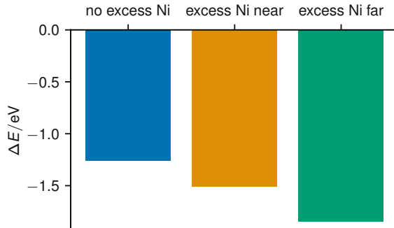
FIG. 1: The energy differences per supercell on dimer formation from a system containing oxygen holes in three cases: no excess Ni (i.e the same energy difference as presented in figure 3 in the main manuscript) and then two additional structures which both contain an excess Ni relative to the first case. In one case, the excess Ni is placed in an octahedral interstitial site near the oxygen holes/dimer, and in the third case it is placed far from these species. In all cases, dimerization is an exothermic process.
